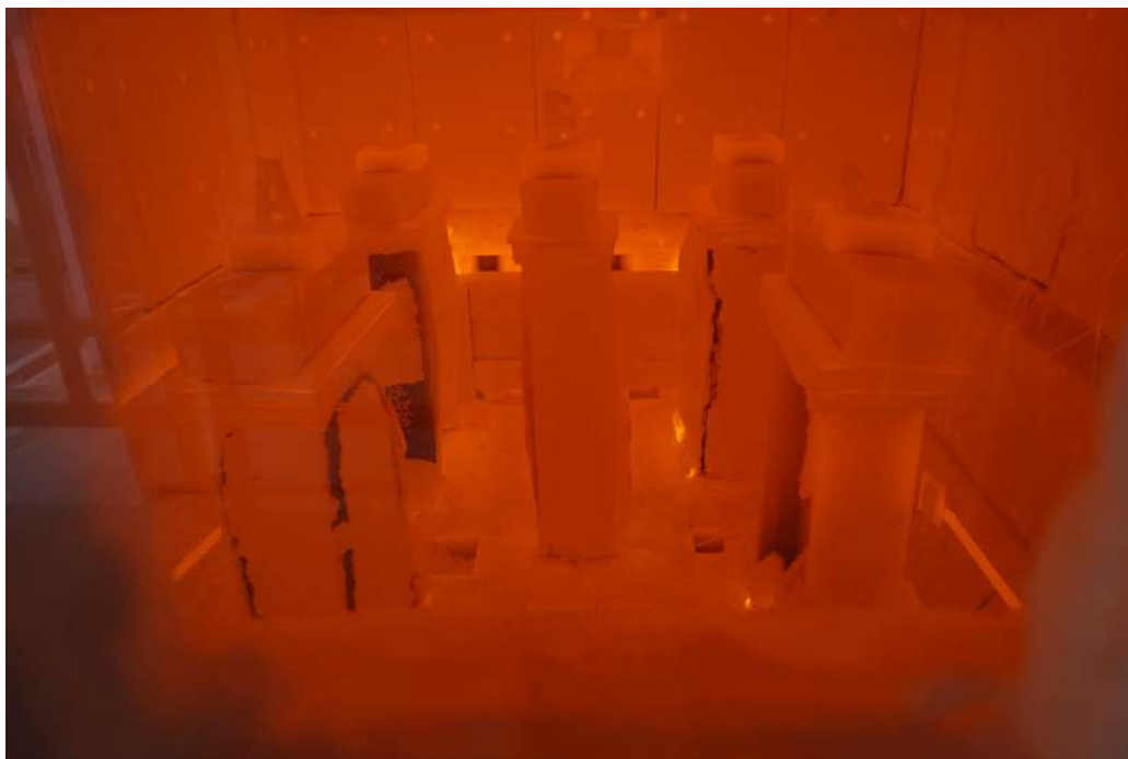
Photo 9: Specimen after 95 minutes of test. (Test terminated)
