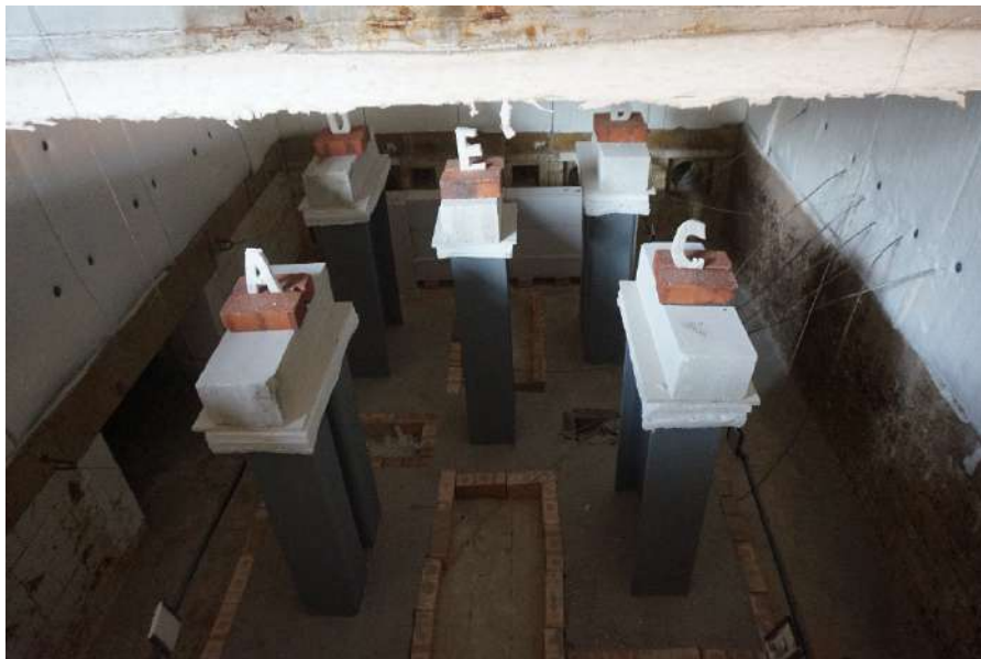
Photo 3: Specimen arranged in furnace.
