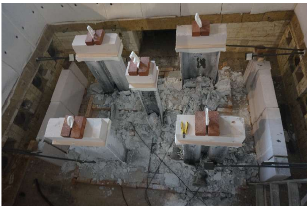
Photo 10: Specimen 12 hours after test termination.
