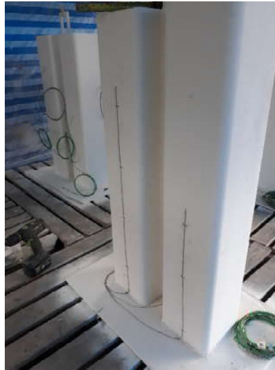
Photo 1: Steel section during specimen thermocouple installation.
